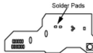
Figure 1. APC PCB, ESD Solder Points
