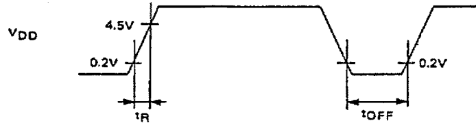
Fig. 8 Power on reset
