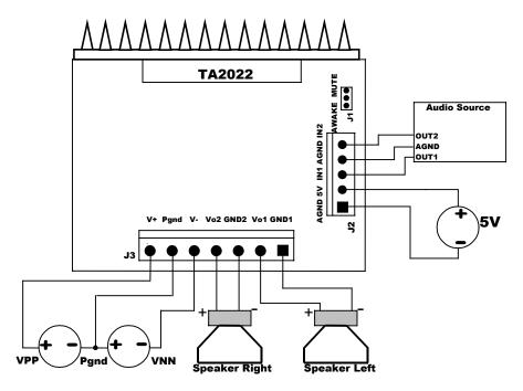
Three external power supplies are required to operate the RB-TA2022: VPP, VNN (referenced to Pgnd), and 5V (referenced to Agnd). The VPP and VNN form a split rail supply referenced to Pgnd. The 5V ground (Agnd) must be kept separate from the VPP and VNN ground (Pgnd). Agnd and Pgnd are joined at a common point on the RB-TA2022 near headers J2 and J3.
